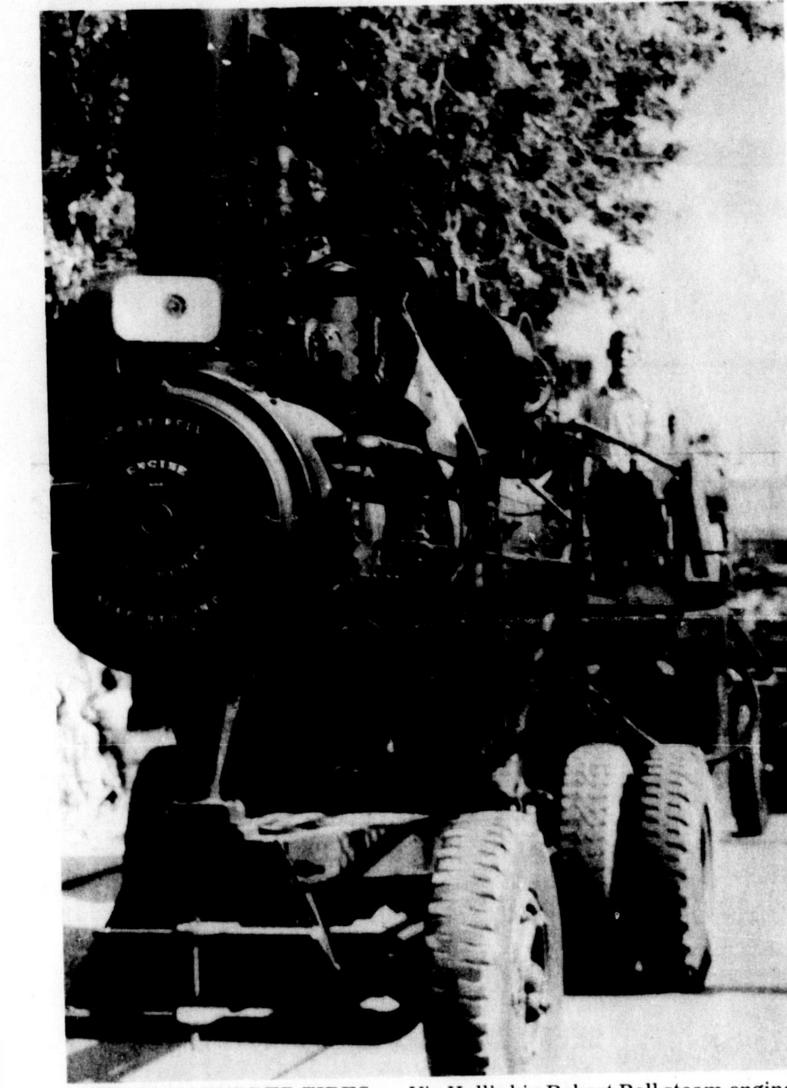
STEAM ON RUBBER TIRES ... Vic Hall's big Robert Bell steam engine is a stationary, mounted on tires for use in parades.
