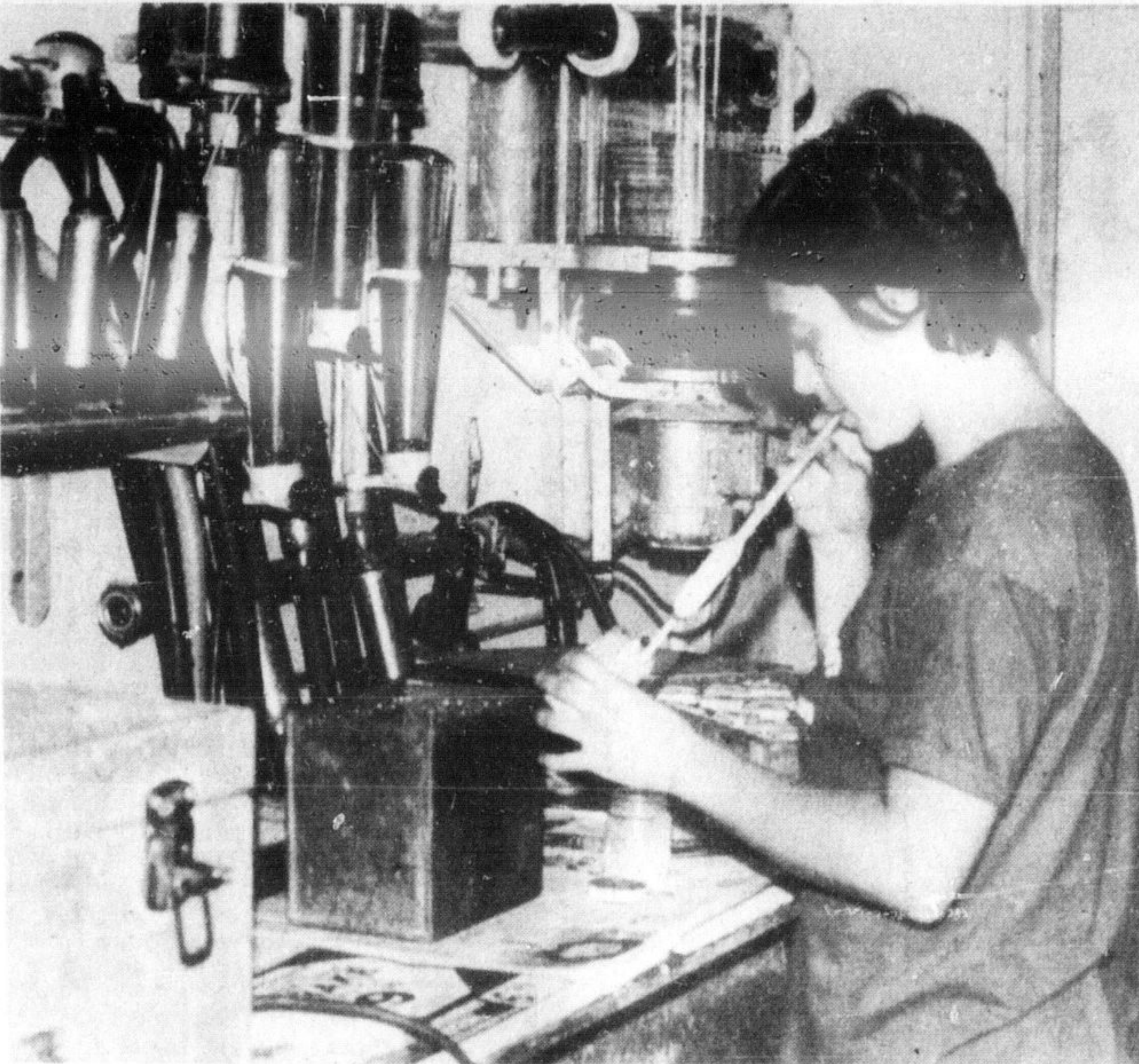
PRECISION is important when testing butterfat levels in milk for federal government records. This specially marked straw tube device ensures R.O.P. tester Sheila Armstrong that exactly 17.6 ml of milk are mixed with 17.5 ml of sulfuric acid—every time. When the mixture has been centrifuged for five minutes and turns black, Sheila adds hot water and watches the butterfat rise.
