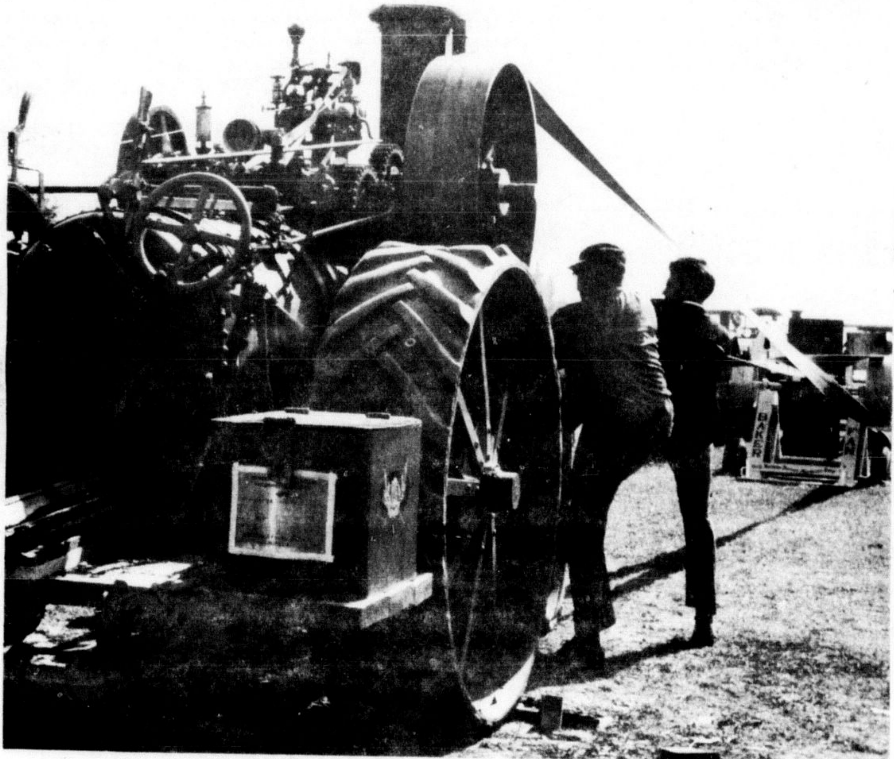
ERNIE ALLEN and a helper prepare to test Mr. Allen's 20 H.P. 1907 White engine by attaching it to a Baker fan, "One of the meanest things a man can hook his engine to" as one old timer said. The fan is used to test an engine's strength.
