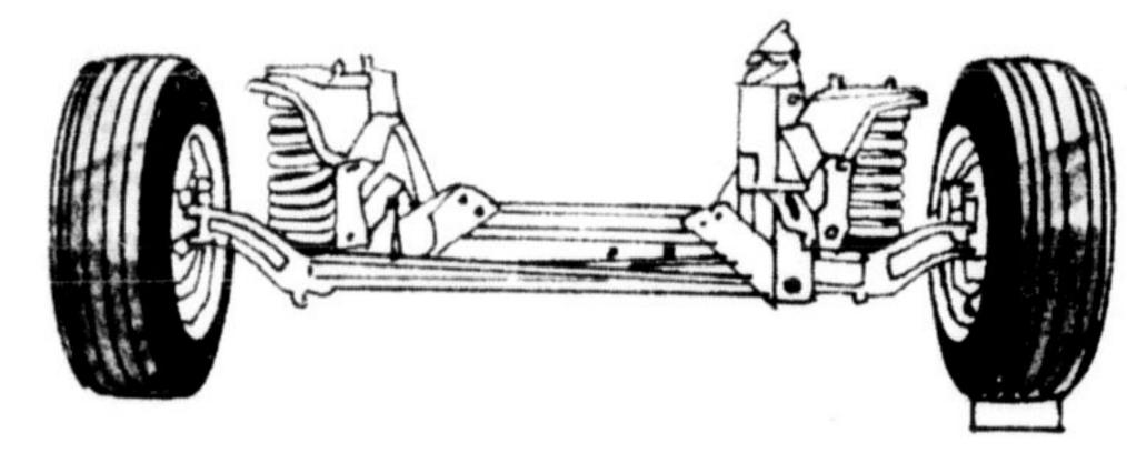
TWIN-I-BEAM FRONT SUSPENSION is a Ford exclusive. Two front axles, each cushioned by a coil spring let each wheel roll over the bumps independently. Each front axle is a forged I-Beam held in place by a rugged I-Beam radius rod to control alignment. This unique suspension absorbs the jolts and bumps of rough roads, and provides smooth stability on the highway.
