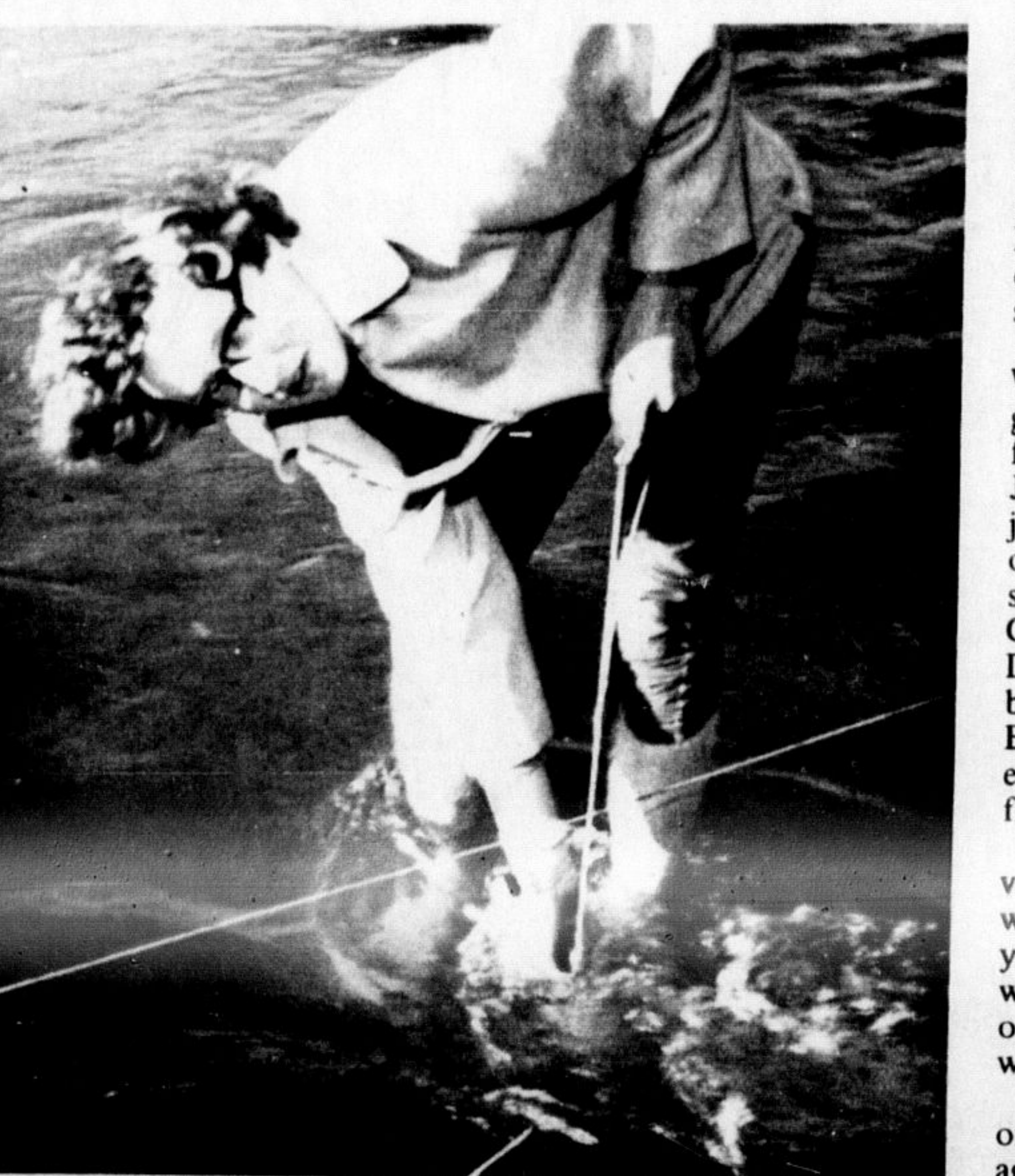
GETTING INTO THE THICK of things, Mats Falk measures the depth of the creek bed at various points. The measurements are fundamental in determining the slope of the river bed and the resulting current. These and similar tests were taken by grade 11 students as part of a study. —(Staff Photo)
