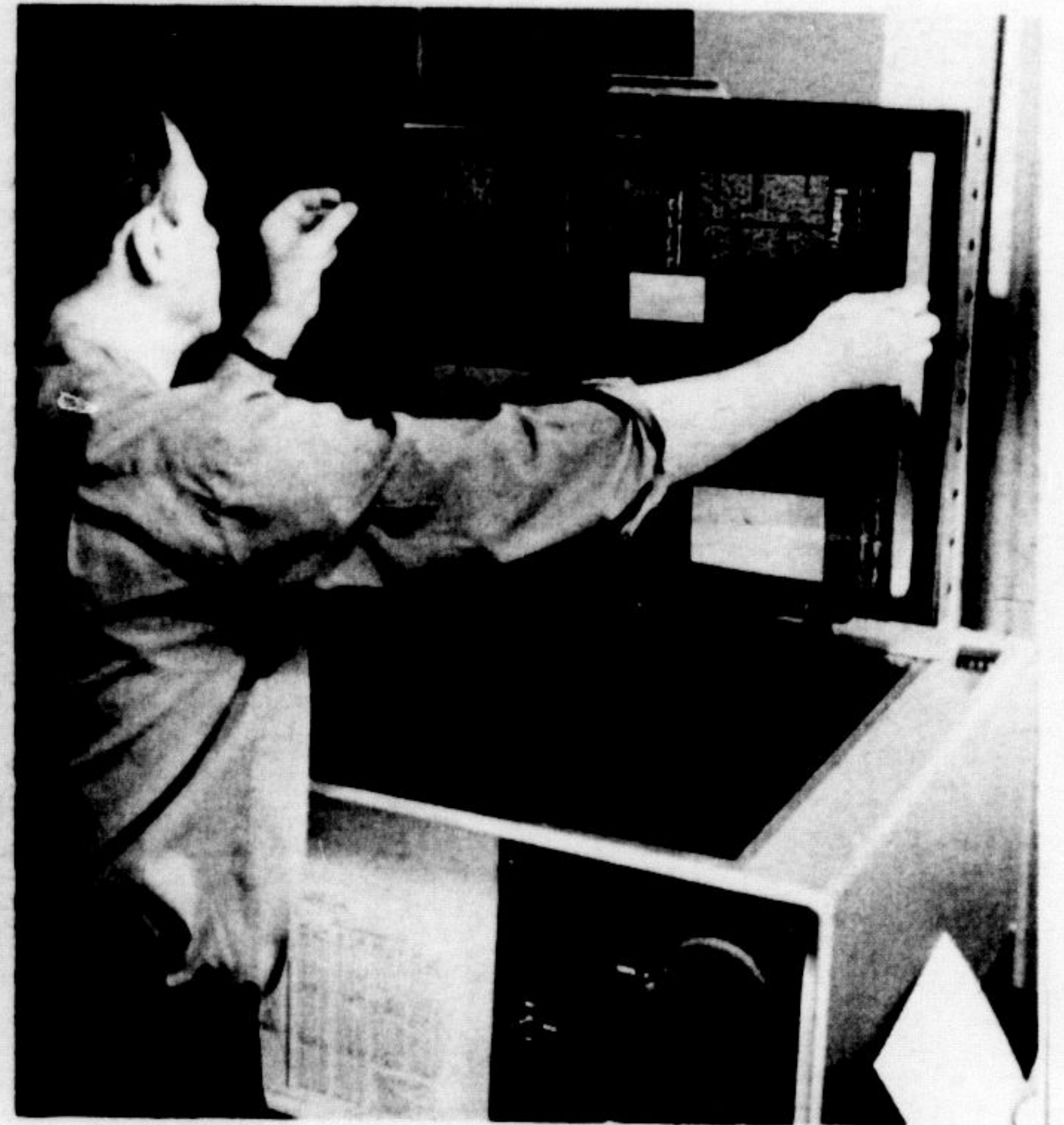
ADJUSTING negative material properly in the back of the vertical camera is important to the final product. The full size negative is an exact reproduction of the pasted-up page.
