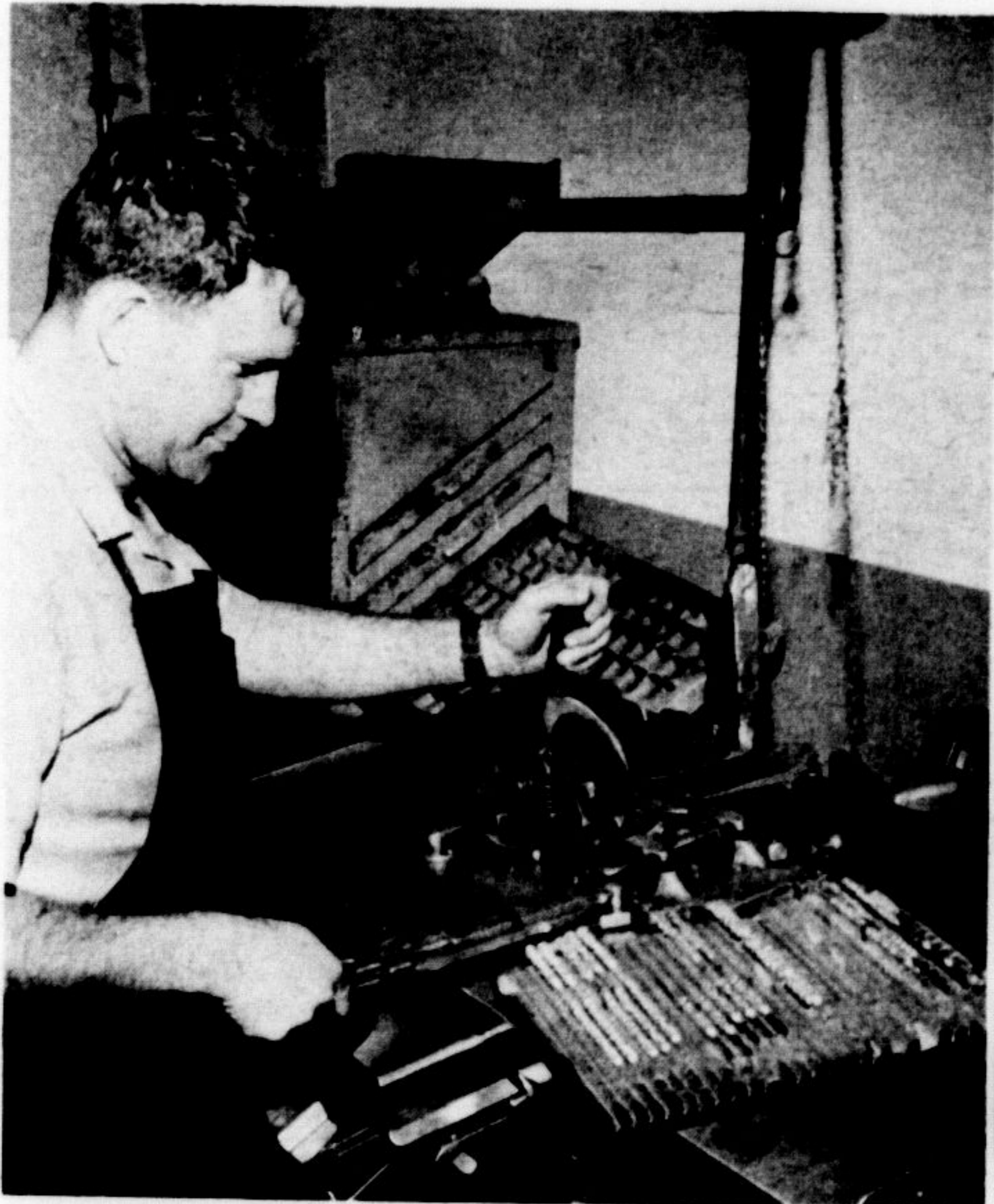
A LUDLOW casts the headlines and larger lines of type in the paper. John Cunningham is shown with the assembled molds preparing to form a line from molten metal.
