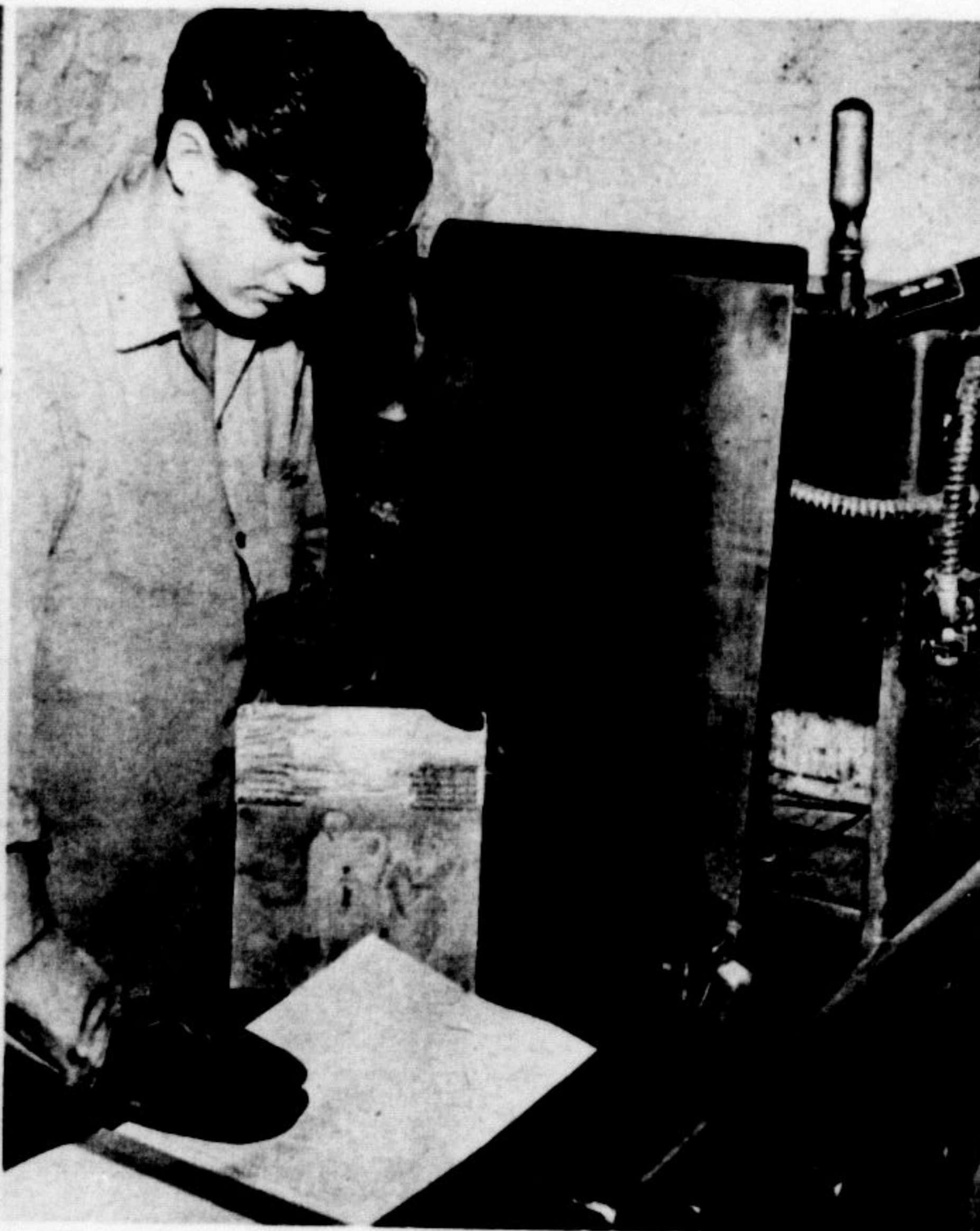
CASTING from a paper mache type of mold, John MacNabb lifts the solid metal printing plate that is produced. In letterpress this would be inked and printed directly.
