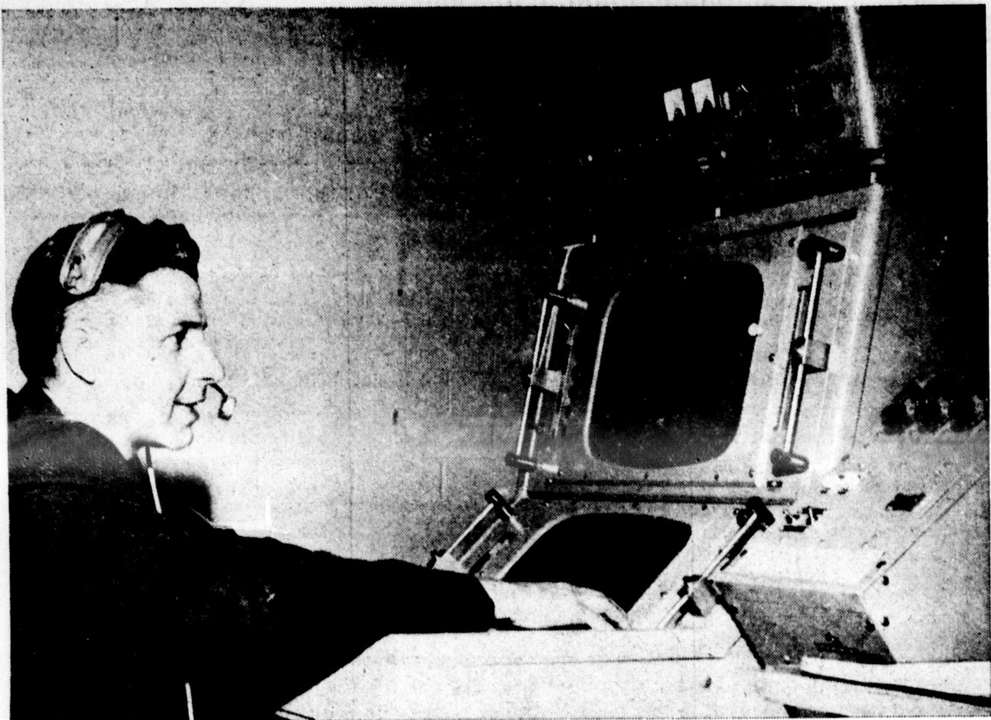
CLAY JUBB OF MILTON, one of three Miltonians working as air traffic controllers at Toronto International Airport at Malton, is shown during a "talkdown" session on the Ground Control Approach console. He follows incoming planes on the two radar scopes in front of him, relaying verbal instruction to the pilot to ensure a safe landing.
