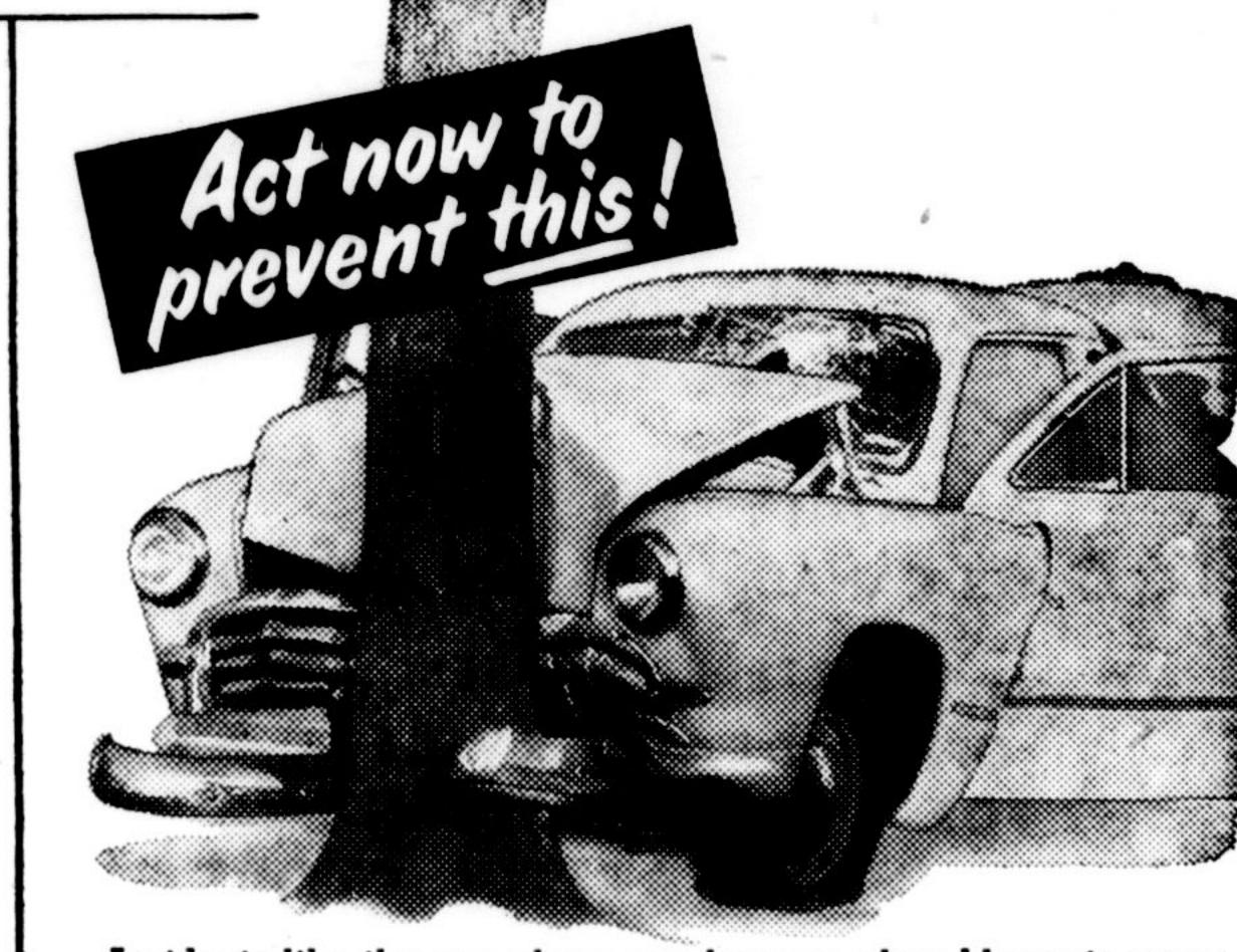
Accidents like the one above can happen when blowouts occurthat's why you owe it to yourself to find out about the extra protection in B. F. Goodrich LIFE-SAVER Tubeless Tires. Most blowouts are caused when the inner tube explodes through weakened or broken cords. But, because it has no inner tube, a LIFE-SAVER Tire changes a sudden, dangerous blowout to a safe s-s-s-slowout allowing you ample time to stop your car safely, with perfect control.
