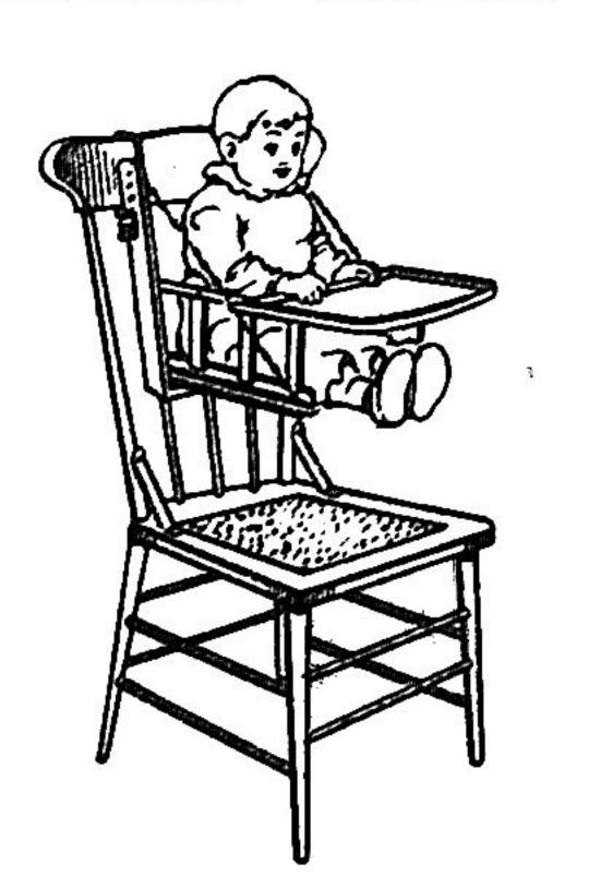
at the top hook over the back of the larger chair. A table is removably fastened on the arms of the baby's chair and answers the double purpose of providing a place for baby's tray , and holding the arms in upright position. This same seat can be used as the seat of a swing by attaching it to chains suspended from ceiling or
