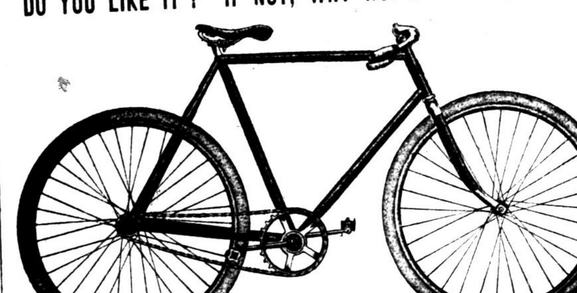
1898 CAPITALS have all the up to date points of advantage that can be desired, including Flush Joints; Internal Seat Post and Haudle Bar Binders; Arch Crown; Low drop Crank Hanger; Two piece Crank, and no Cotter Pins; Dust Proof Bearings; Ball retaining and Felt Washers. Tr.
