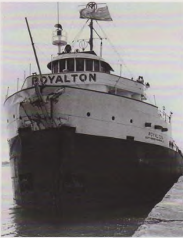
Here, courtesy Ron Beaupre, is ROYALTON at Port Colborne showing the bow damage sustained in the June 1959 collision with MONROVIA.
