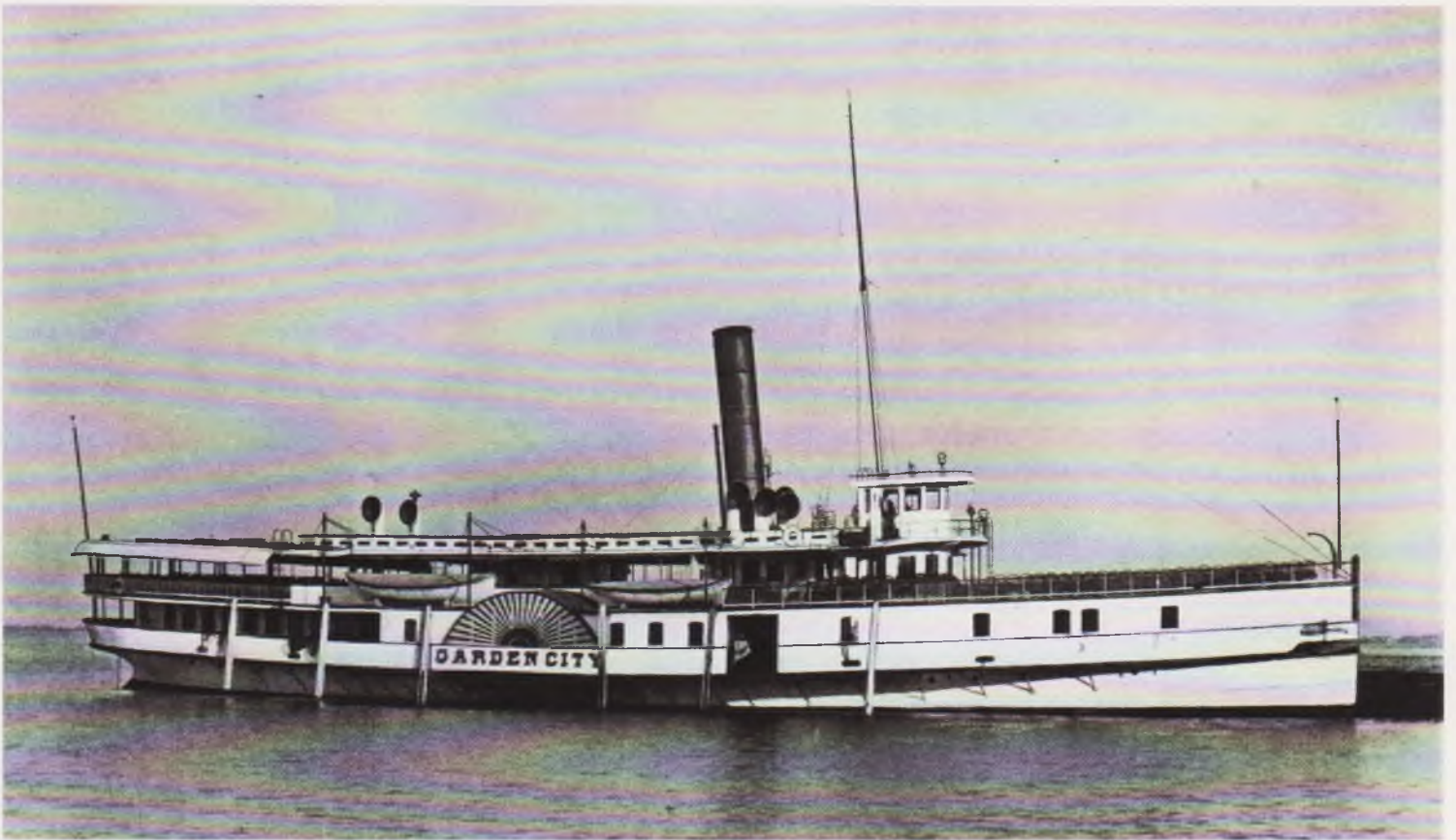
An early photo shows GARDEN CITY before the texas cabin was added on the hurricane deck.
