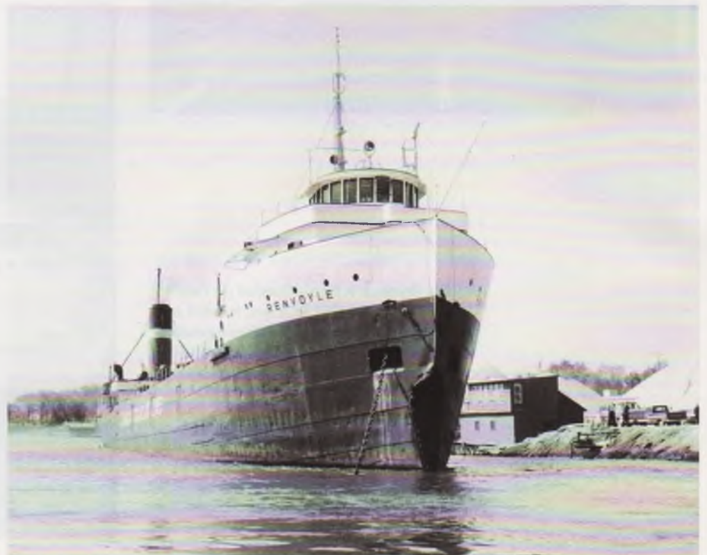
It is June 1, 1967, and RENVOYLE lies at anchor in the St. Clair River off Port Huron after sinking SYLVANIA. Note her bow damage.
