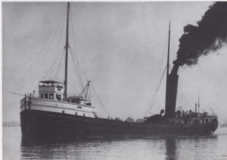
Pesha photo, courtesy Rev. Peter Van der Linden, shows MAJOR with her old masts cut down, before they were replaced with steel pipe spars.
