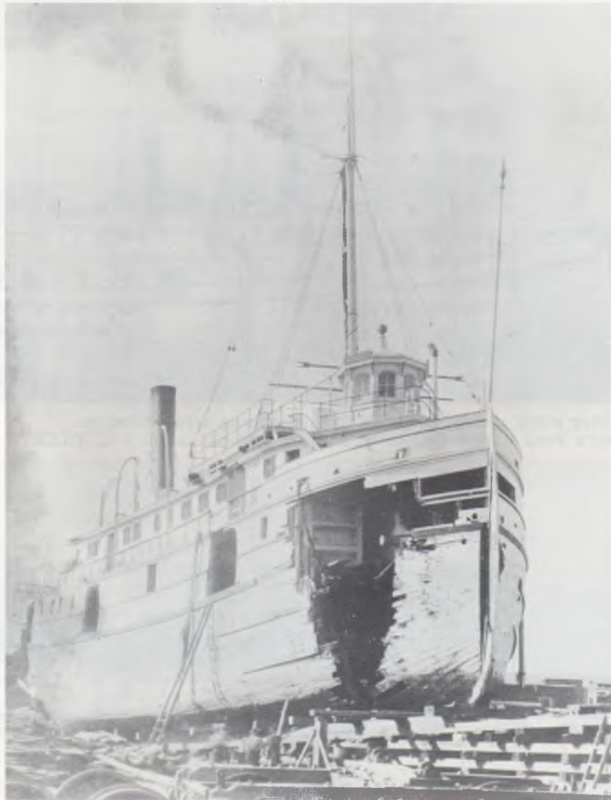
This spectacular photo shows OCEAN on Rathbun's marine railway at Deseronto after her June 7, 1894, collision with the barge KENT.
