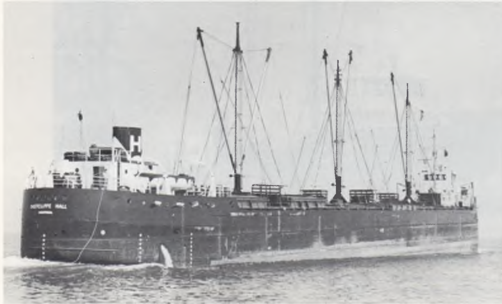
(Above and left) The lengthened EASTCLIFFE HALL was outbound at Toronto's Eastern Gap when photographed by the Editor on July 29, 1960. Note the full lines of her cruiser stern.
