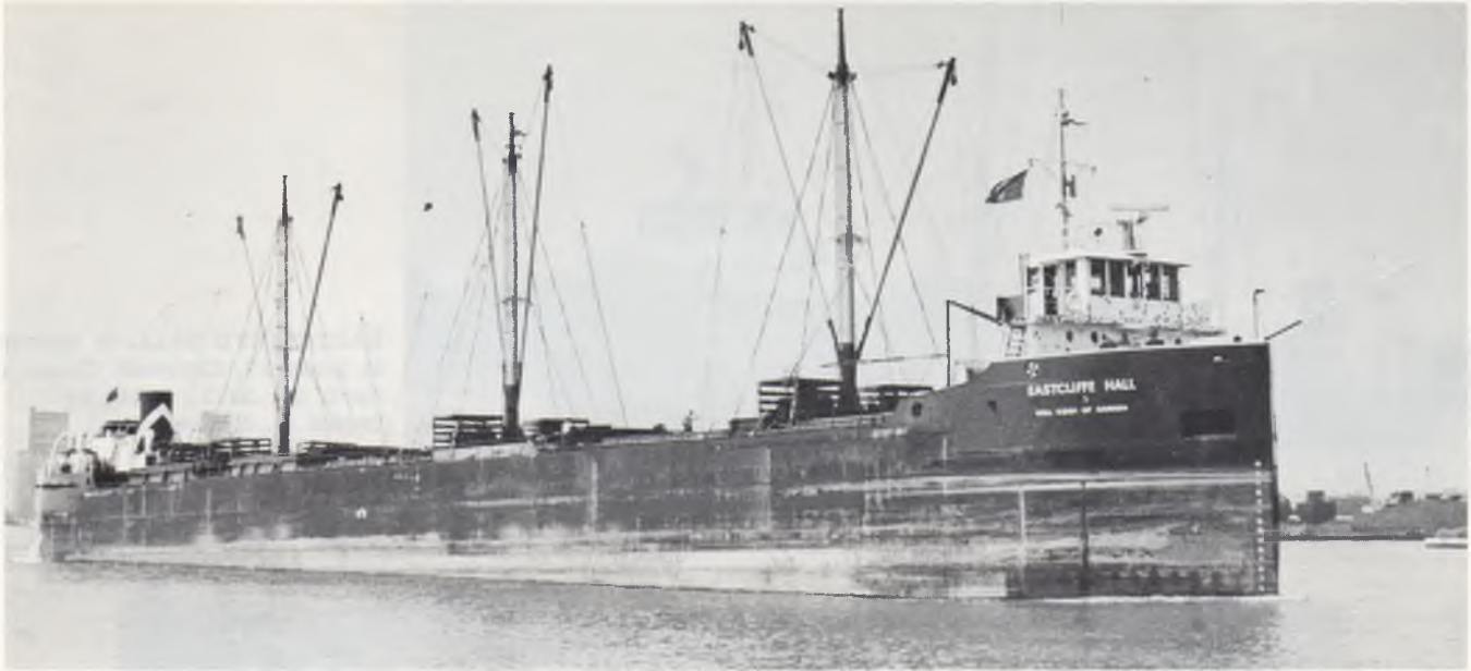
(Above and left) The lengthened EASTCLIFFE HALL was outbound at Toronto's Eastern Gap when photographed by the Editor on July 29, 1960. Note the full lines of her cruiser stern.
