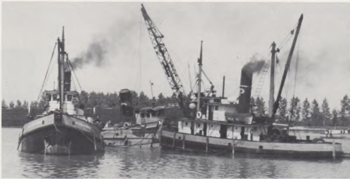
This James M. Kidd photo caught SALVAGE PRINCE (left) and S.A. QUEEN (right) lifting DALHOUSIE ROVER from the waters of the Welland Canal.
