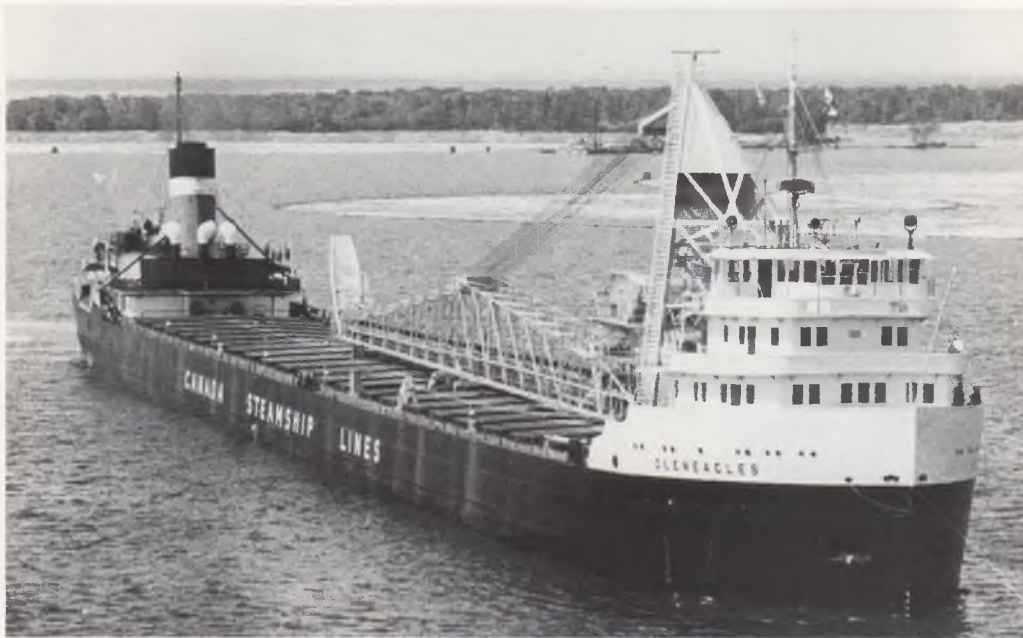
The tall bridge structure of GLENEAGLES helped to overcome the aesthetic damage done by her self-unloader conversion. Photo by John Vournakis.
