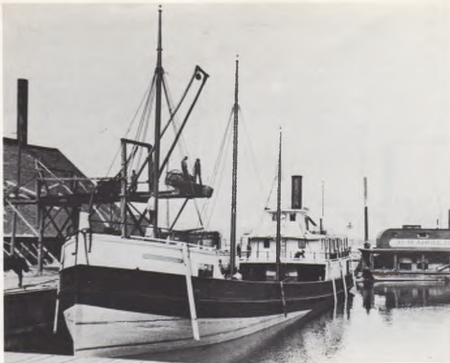
A very early photo of JUNO, courtesy Ron Beaupre, shows her as a "Rabbit", with three masts, and her pilothouse and cabins aft.
