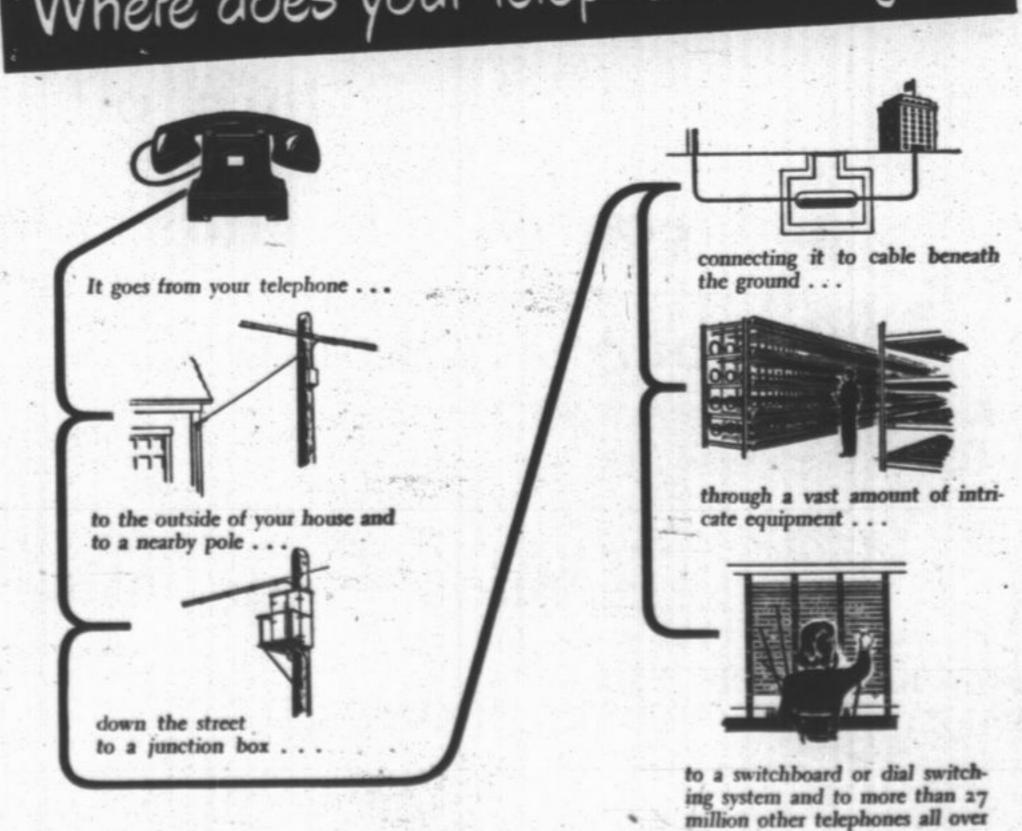
A telephone instrument is only a small fraction of the equipment needed to provide service for each telephone.
