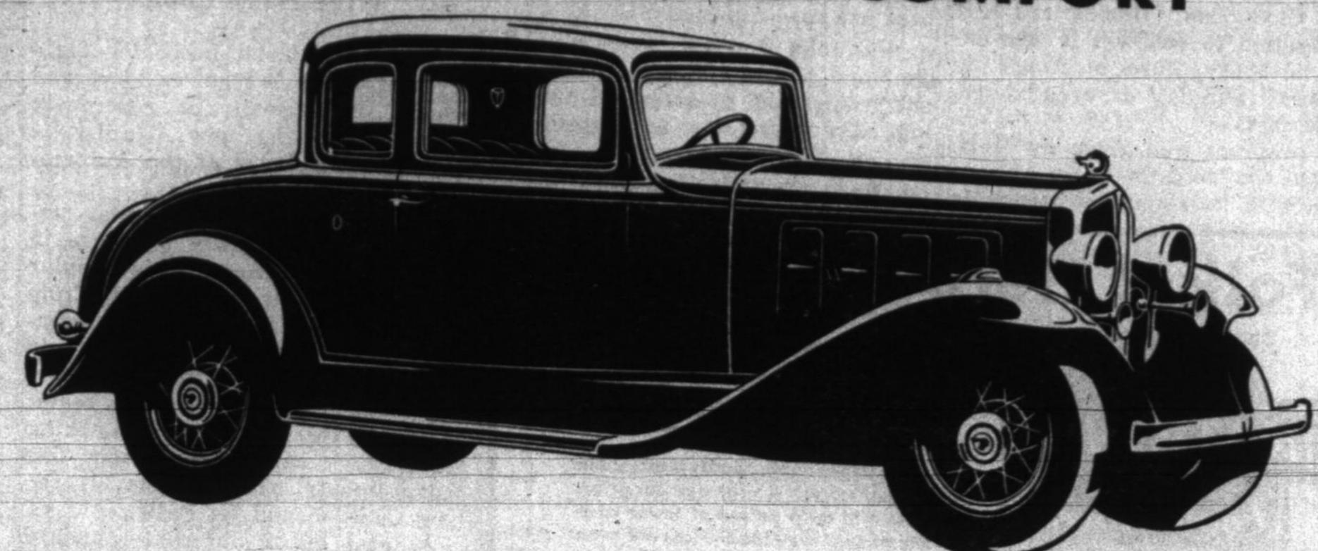
With Ride Control—the newest development—you adjust shock absorber action to rough or smooth roads, by touching a button on the dash. Then, there is rubber cushioning at 47 chassis points—a remarkably complete system which insulates the motor and other mechanical units from the frame, and the frame from the body. The long wheelbase assures road-steadiness, and the enclosed, self-lubricating springs further promote easy riding.
