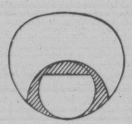
This sketch is shaded to show the blind area and useless parts of the old-type Kryptok bifocals. These blind segment-edges were worse than useless. They tended to blur nearby objects. In UNIVIS the space they occupied added to the distance field.
