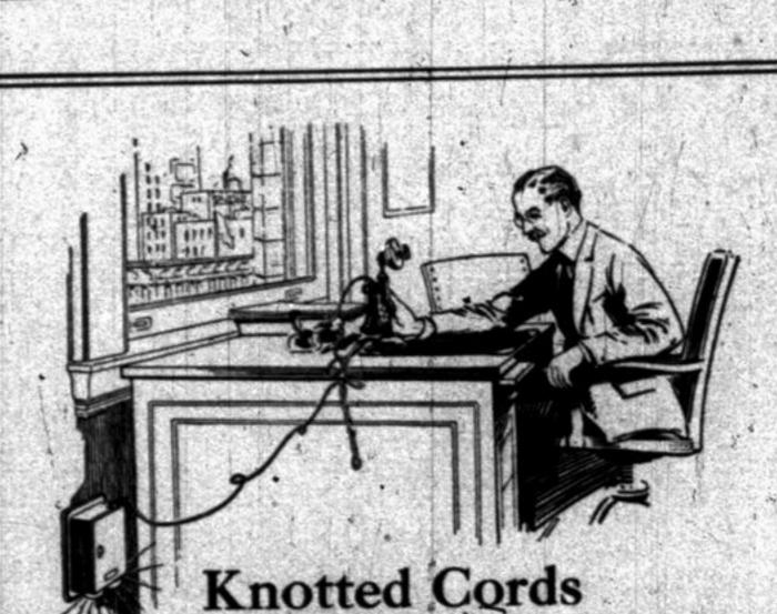
Make Noisy Lines The cloth-covered cord which connects your telephone instrument with the bell box and the cord running to the telephone receiver are each made up of a number of fine wires covered with light insulation. If these cords were not made in this way they would not be flexible. They are necessarily delicate
