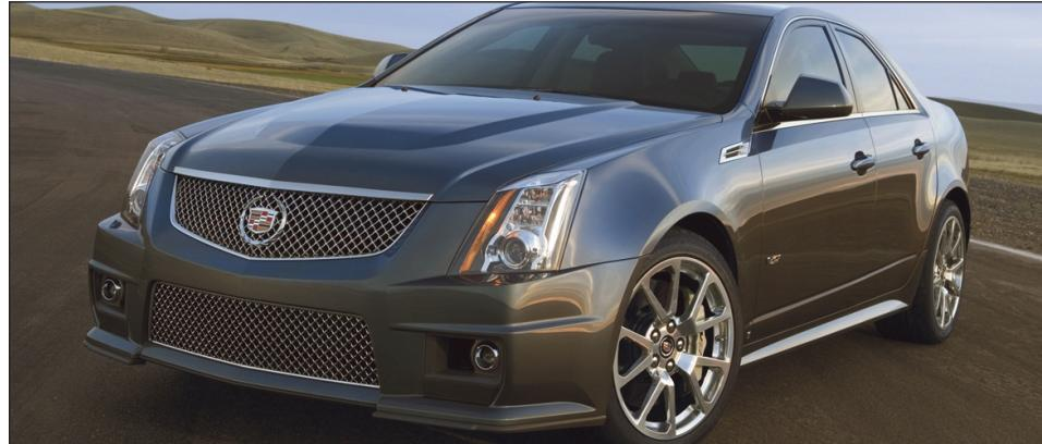
Testing of the 2009 Cadillac CTS-V has shown its produces 556 hp with a 0-60 mph acceleration time of 3.9 seconds making it the fastest V8 production car in the world.
