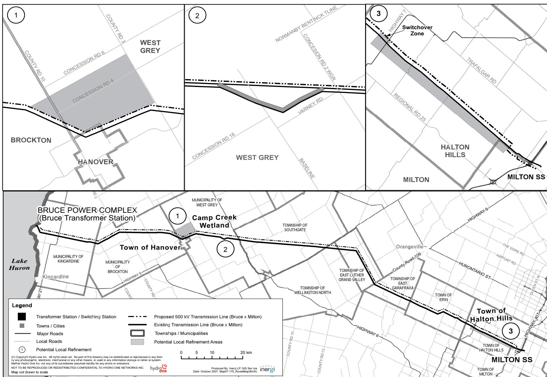
Hydro One Networks Inc. ("Hydro One") is proposing to build an approximately 180 kilometre double-circuit 500,000 volt (500 kV) transmission line on a widened existing transmission corridor from the Bruce Power Facility ("Bruce") in Kincardine to Hydro One's switching station in Milton ("Milton"). The Ontario Power Authority identified and confirmed the need and route for the new transmission line earlier this year.
