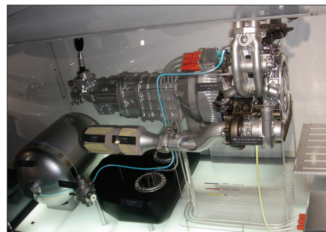
This display shows how the gasoline and hydrogen rotary works.
