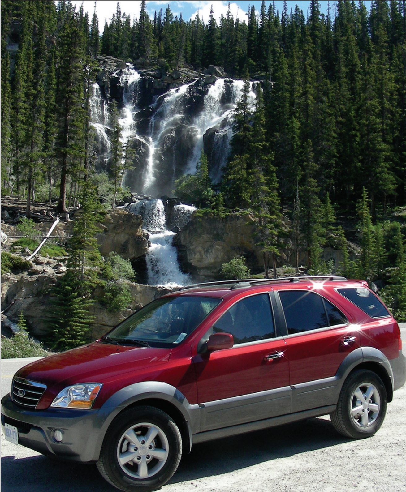
The 2008 Kia Sorento is outwardly only slightly changed but everything under the skin is new, like a choice of two V6 engines and a full body on frame with nine steel cross members. Photo by Jim Robinson
