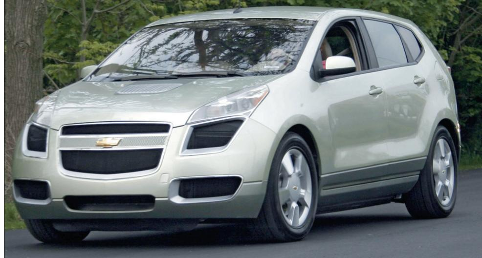
The Chevy Sequel recently set a new record as the first electrically-driven fuel cell vehicle to achieve 300 miles on one tank of hydrogen, in and out of traffic on public roads, while producing zero emissions.
