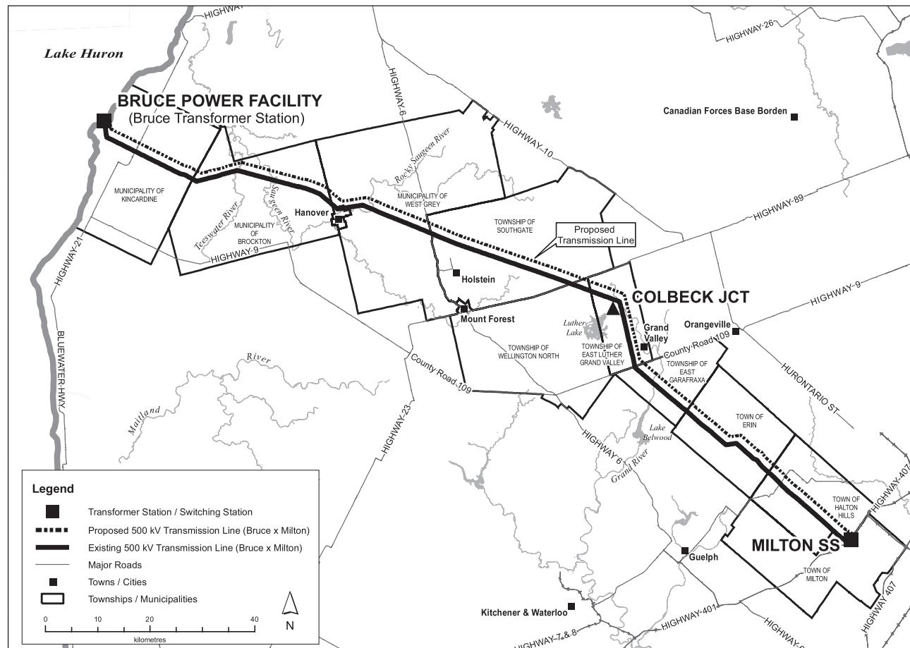
Hydro One Networks Inc. ("Hydro One") has initiated a Project under Ontario's Environmental Assessment Act (the "Act") to build an approximately 180 kilometre double circuit 500,000 volt (500 kV) transmission line on a widened existing transmission corridor connecting the Bruce Power facility ("Bruce") in Kincardine to Hydro One's switching station in Milton ("Milton").
