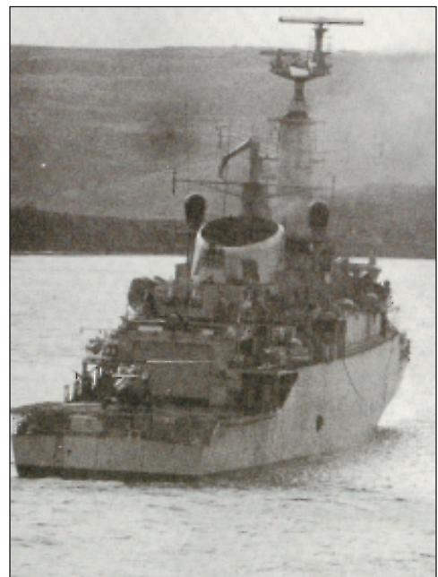
HMS Antelope, with the relatively innocent-looking one metre hole in the side of its hull, moved to a safer location after sustaining two bomb hits from an air attack.
