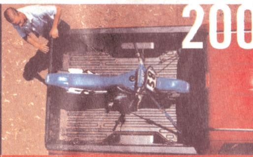
Fibre-reinforced sheet-moulded composite bed
