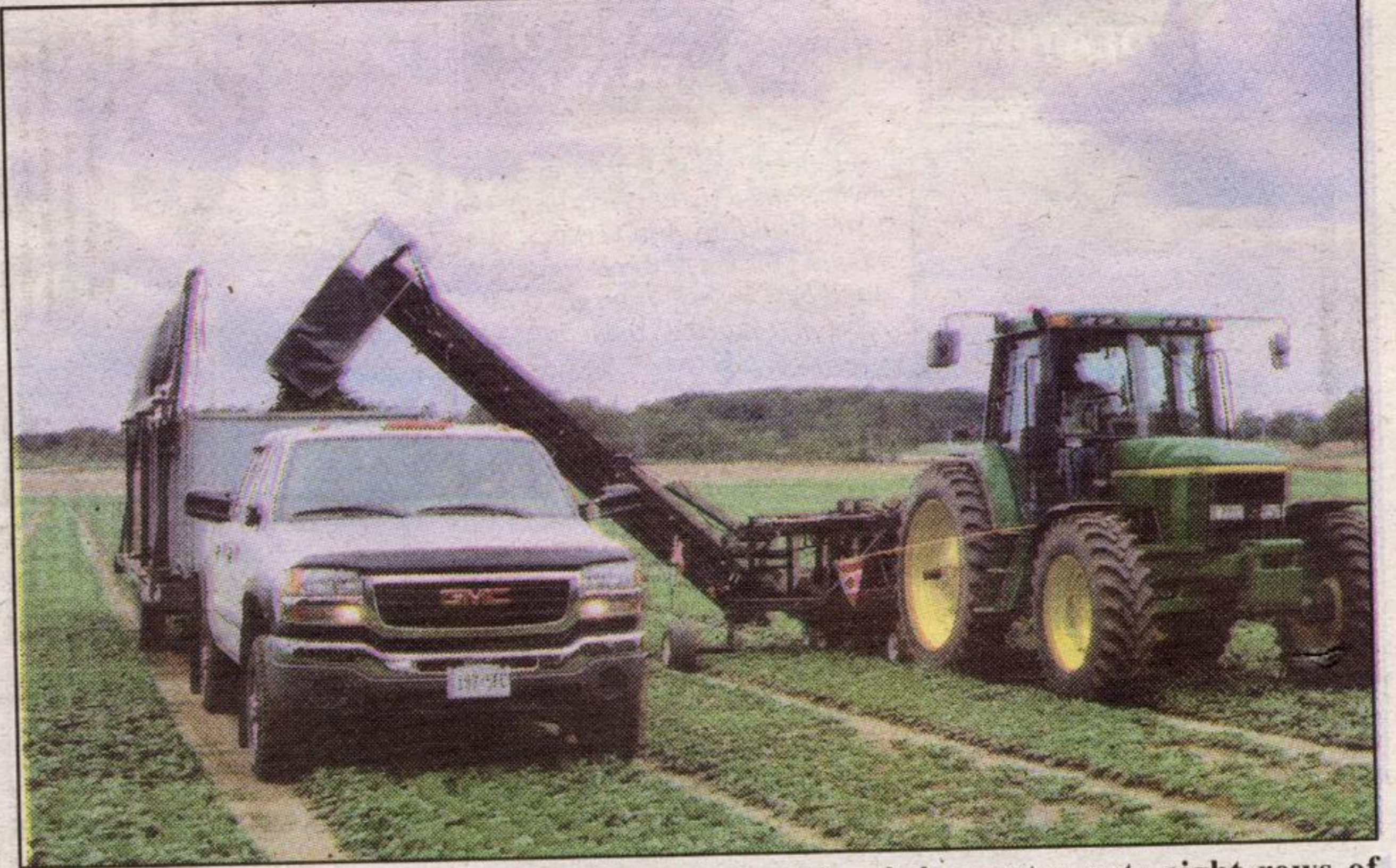
HARVESTING THE CROP: This homemade spinach harvester cuts eight rows of spinach at a time. The spinach is then poured via conveyor belt into the bins, which are hauled to the on-site packing facility. Photo by Rebecca Ring
