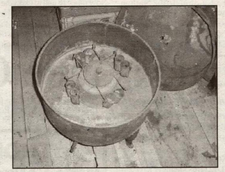
It has a wooden floor and a crank to turn the centre wheel. Turning this wheel causes the cups to tip their contents into the drum. If you have any ideas about what could have been made or processed in this intriguing invention of yesteryear, call The New Tanner at 519-853-0051 and let us know.
