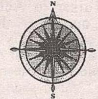
USED TO DETERMINE DIRECTION, A MARINER'S COMPASS HAS A MAGNETIC NEEDLE THAT TURNS TO ALIGN ITSELF WITH THE MAGNETIC NORTH AND SOUTH POLES. THIS DEVICE PROBABLY FIRST WAS USED BY EUROPEAN SEAMEN IN THE 12TH CENTURY.
