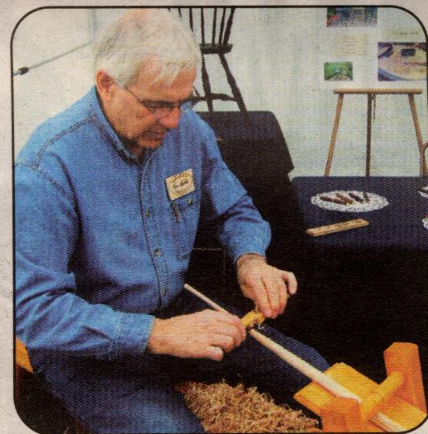
Ken Keates using a spoke shave to make a spindle for a chair back.
