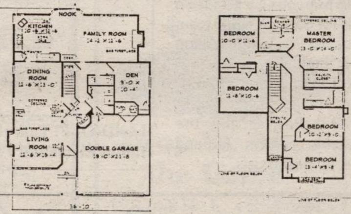
MAIN FLOOR PLAN 1246 SQ. FT. UPPER FLOOR PLAN 1115 SQ. FT. TOTAL FLOOR AREA 2361 SQ. FT.
