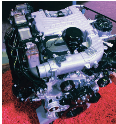
The heart of the 2016 Nissan Titan is its Cummins-sourced 5.0-litre two-stage turbo diesel engine putting out 310 hp and 555 lb/ft of torque.
