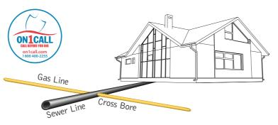
A damaged gas line can result in a serious safety risk.
