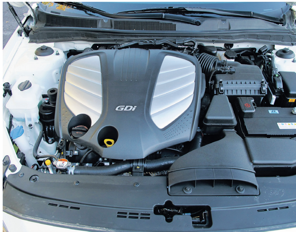
The 2016 Kia Cadenza is powered by a 3.3-litre direct injection V6 with 293 hp and 255 lb/ft of torque driving the front wheels through a six-speed automatic transmission with sequential manual shift mode.
