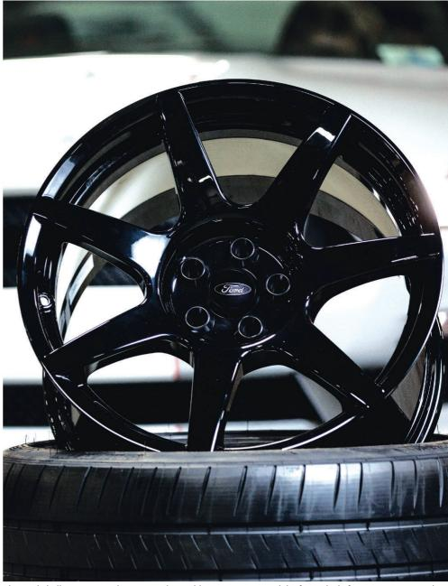
The Ford Shelby GT350R is the most track-capable Mustang ever and the first vehicle from a major automaker to offer carbon fibre wheels as standard equipment. In early testing with benchmark vehicles, prototype wheels showed significant potential - improving suspension response times, chassis dynamics, steering feel and ride quality.
