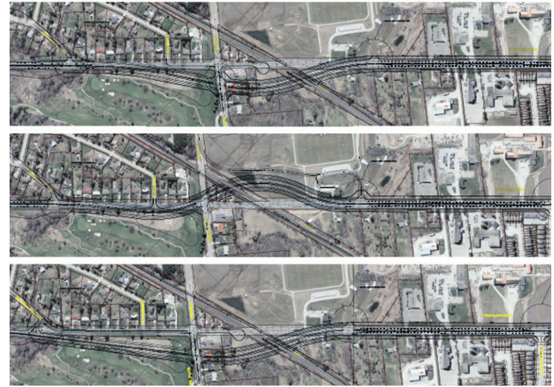
Alternatives 1A, 1B and 1C show different options between considered on Trafalgar Rd. at the Maple Ave./17 Sideroad intersection.
