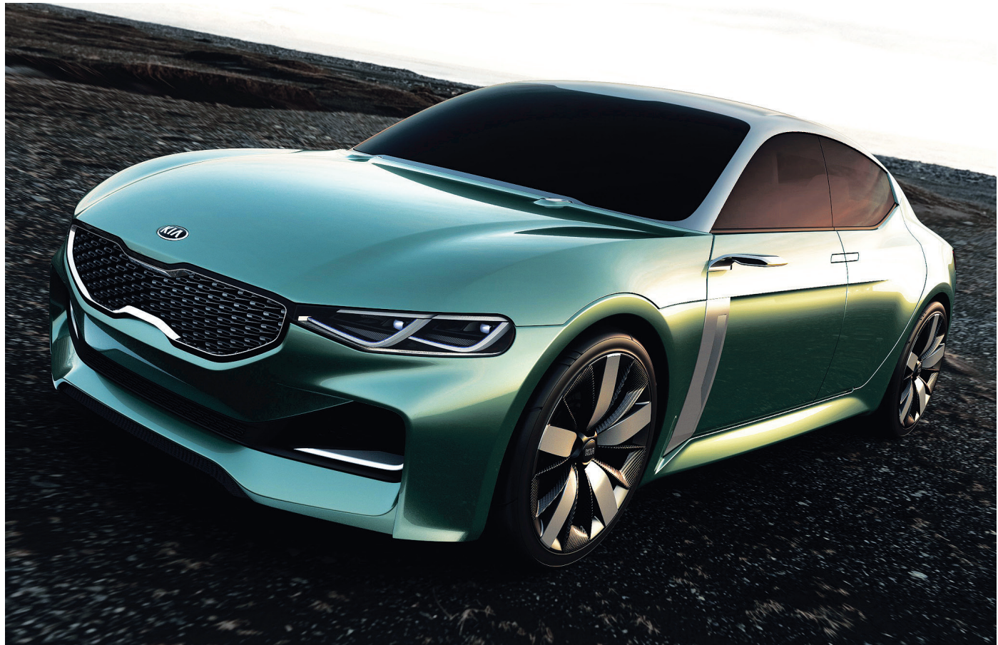
Coupe style was selected for Kia's latest concept, the Novo, with 1.6-litre turbo direct injection four-cylinder engine and seven-speed dual clutch transmission.
