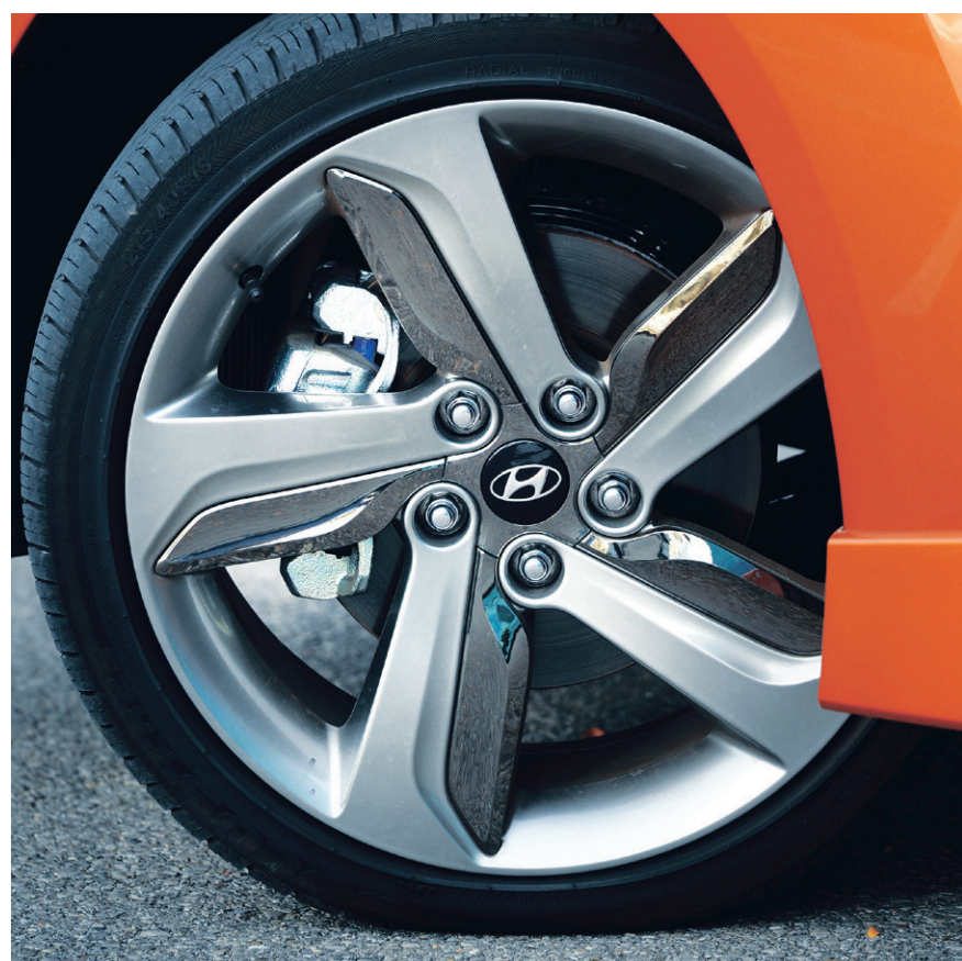
The Veloster Turbo's bigger 18-inch wheels mount lower profile, performance-oriented P215/40/VR18 tires.
