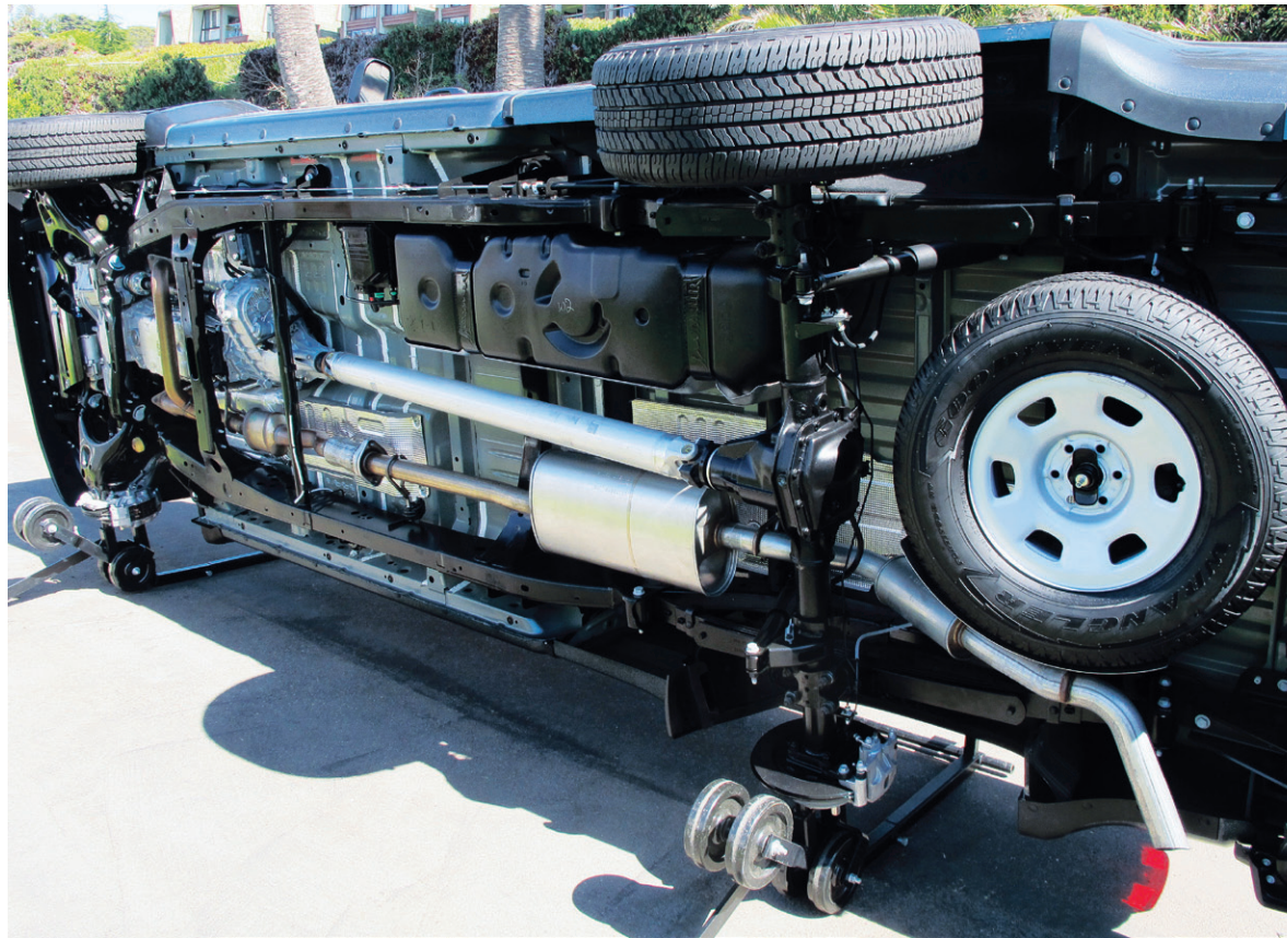
The Colorado/Canyon are fully box-framed with shear-style and compression body mounts. Suspension is a coil over strut system with large diameter, hollow stabilizers bars and twin-tube shocks with two-stage leaf springs and a Hotchkiss-style solid rear axle.
