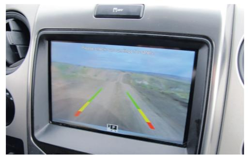
The Ford Raptor also has a front facing camera that allows the driver to see what is below his field of view such as boulders or in this case, coming down with the standard Hill Descent Control engaged.
