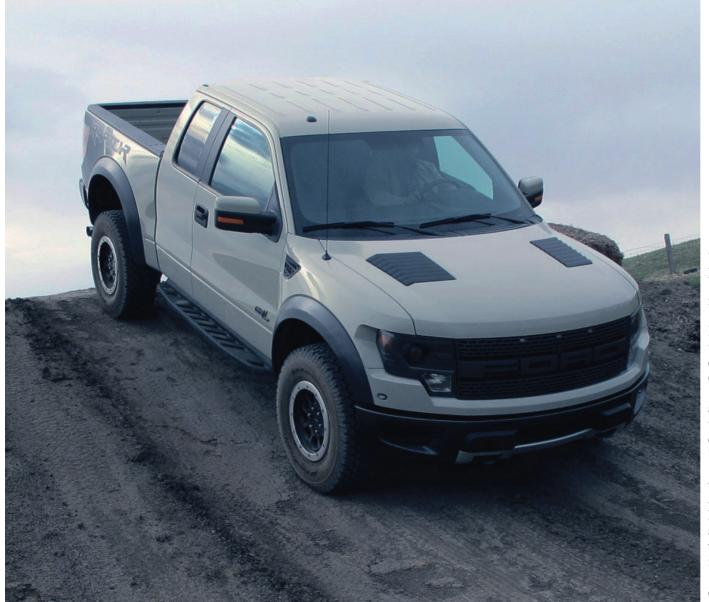
When it comes to going down steep inclines, standard Hill Descent Control is what you want. The Raptor also comes with stack for 2H, 4A, 4H and 4L (two-wheel high, available "beadlock" rims (shown) that lock the tire to the special forged wheel to prevent them rolling off when air pressure all-wheel-drive, four-high and four-low). has been reduced to extreme grip conditions.
