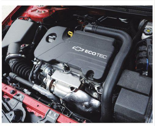
Most trim levels, like the LT, harness a new standard turbocharged 1.5-litre Ecotec four-cylinder with VVT and stop/start technology (166 hp, 184 lb/ft). Fuel economy is rated at 8.7/6.3L/100m (city/hwy).
