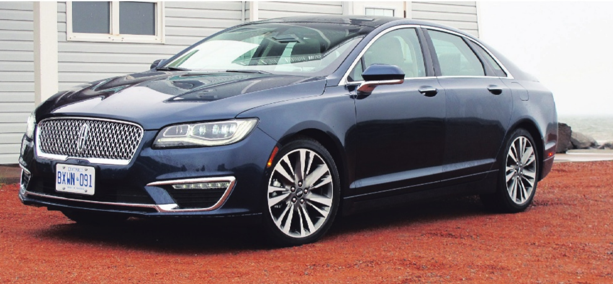
The 2017 Lincoln MKZ (Reserve model shown) gets a new grille and optional LED headlight treatment which unclutters the nose compared to the outgoing model.
