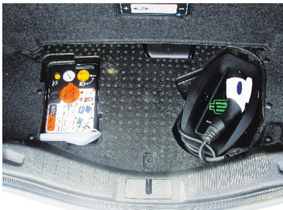
Beneath the cargo floor is the plug-in charger cord and a professional grade tire inflator kit as there is no room for a spare tire on the Fusion plug-in hybrid.
